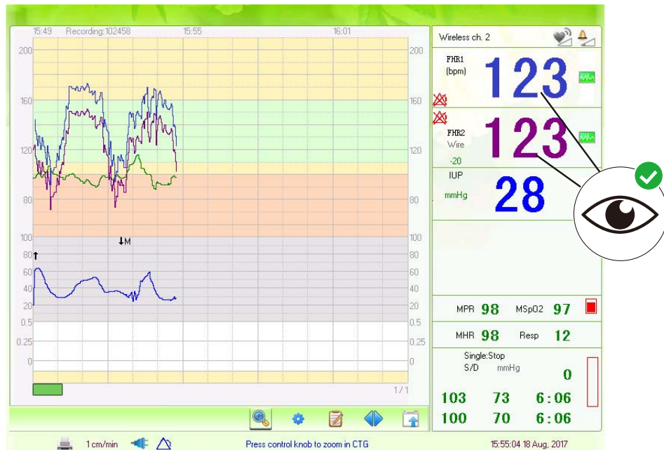
Figure 6:58 Verify that an FHR1/FHR2 value appears on the display
