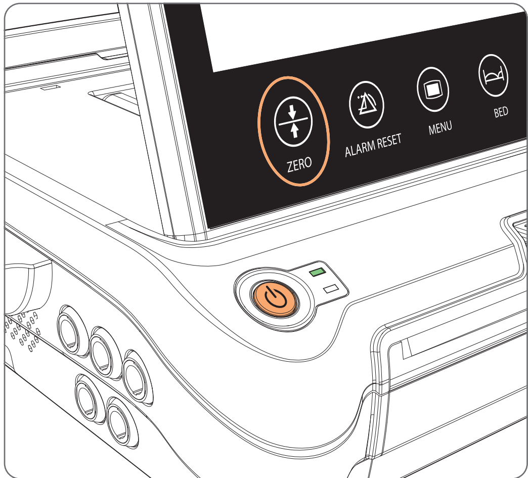
Figure 4:61 Zero TOCO functions using the “ZERO” touch key
