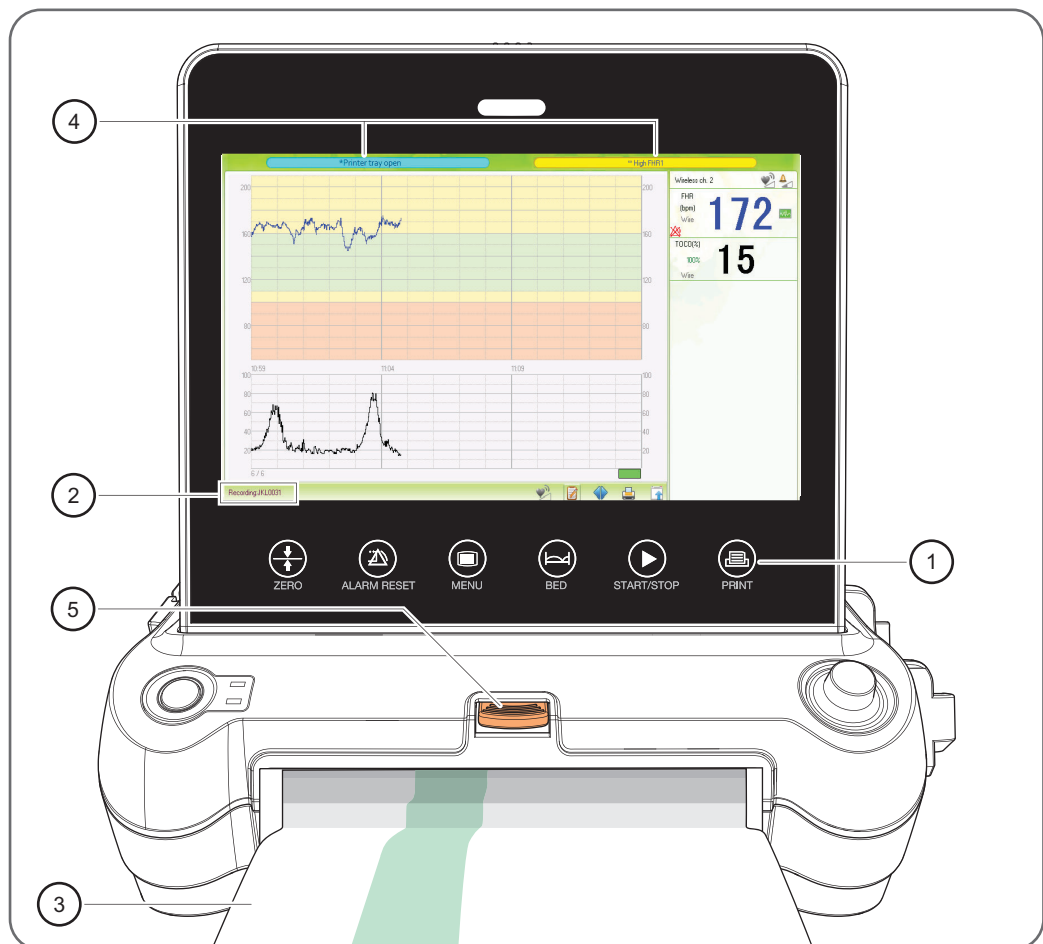
Figure 3:37 View of printer with associated controls
